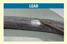
Your Service Line is Lead if: Scratch Test: The scratched area is
