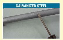
Your Service Line is Galvanized Steel if: Scratch Test: The scratched area remains a dull gray. Magnet Test: The magnet sticks. Tapping Test: You hear a metallic ringing noise when tapping the coin.
